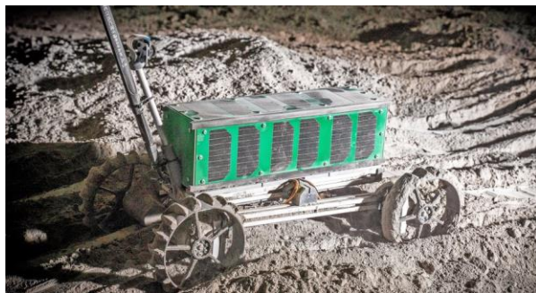
Figure 1 The HiveR rover during a test in an artificial lunar environment. [6]
